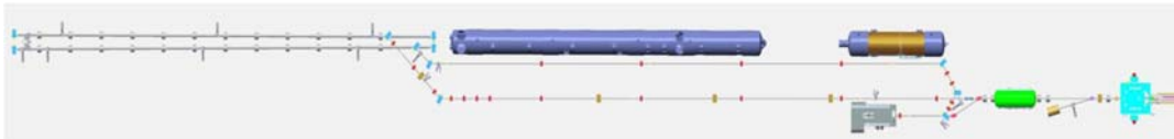
Figure 1: Layout of LEReC in IP2 region of RHIC (from right to left: gun shown with light blue color followed by the SRF 5-cell cavity (green), electron beam transport line, two cooling sections with solenoids, return beam line and beam dump).
