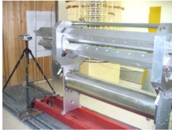
Figure 10: Helical wiggler at the magnetic-measurements stand.
