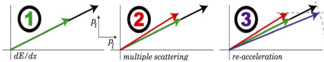
Figure 1: Ionization cooling principle. Green arrow: momentum reduction in the absorber, red arrow: reduction of the cooling effect due to multiple scattering, purple arrow: longitudinal momentum restored in a set of RF cavities.
